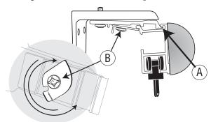
Ceiling mount, double mount and decorative bracket installations use the same mounting clip (93630) and rods attach the same way.
